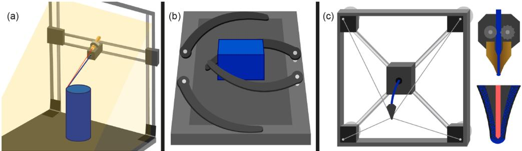
Fig. 3. Three design alternatives for book-shaped 3D printers: (a) remote heating with angled extrusion; (b) lifting the model; (c) a wire-driven delta printer.
