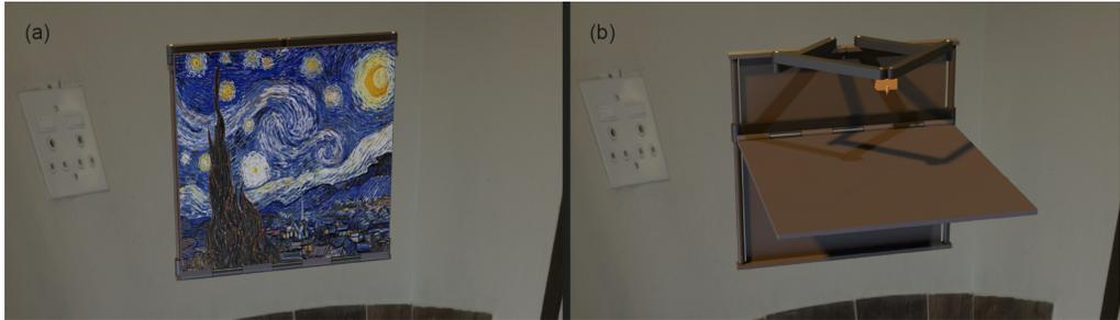
Fig. 1. Fabrication in the living room: (a) the printer acts as decoration while out of use; (b) it unfolds to become a fully functional 3D printer.
