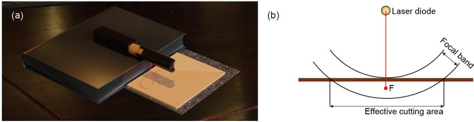
Fig. 2. A pen-shaped laser cutter design: (a) the device can be operated in the living room. (b) Operational limits based on focus requirements for laser cutting.
