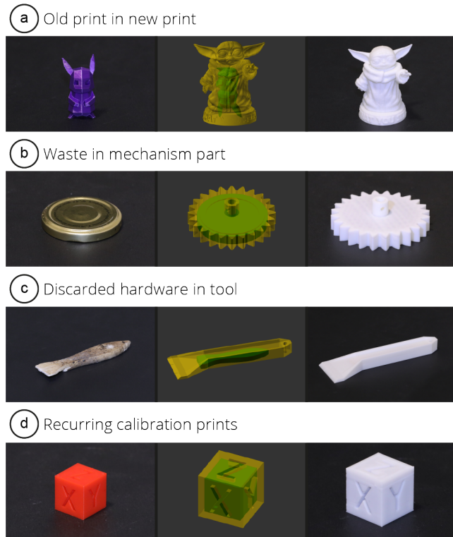
Figure 4: Examples showing scrap, computed mesh, and printed model: (a) an outdated print inside a new one; (b) household waste inside a mechanical part; (c) the broken handle of a hand tool inside another tool, (d) and a recurring print used to calibrate printers inside a bigger version of the same model.
